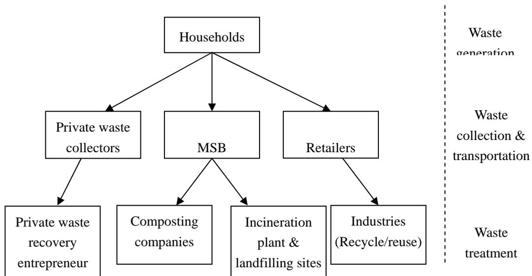
**Fig.5** MSW generation, collection and treatment process in the old city of Ningbo
