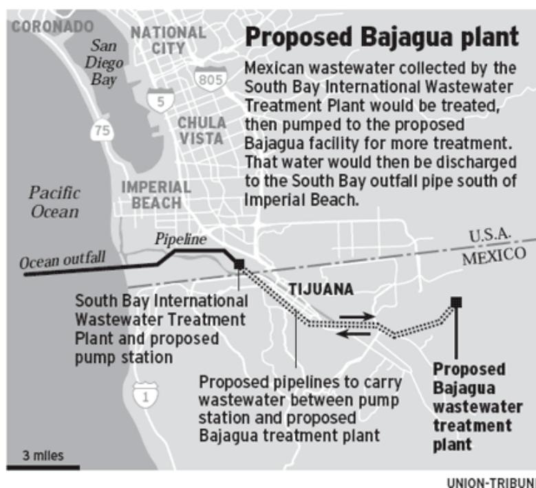
**Figure 6:** Proposed Bajagua plant and pipelines.
