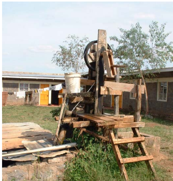
Figure 5: This well, at KIOF, demonstrates how appropriate technology can result in increased efficiency on the farm. This well system is built with recycled wood, a tire, a bucket, and a length of rope. Called the “rope and washer”, it provides the ability to draw water from a well without inputs from outside the farm.
