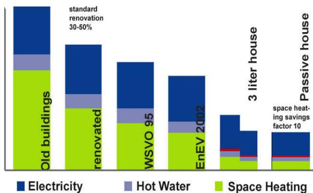
Fig. 12: German energy efficient standards for houses (Schulze Darup 2003)
